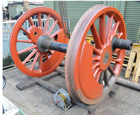
The Driving Wheel Set whilst being painted.
